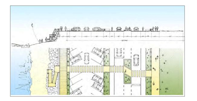
Following the Phase 1 Study, some community members voiced concerns about moving the highway significantly further inland or adding parking on the inland side of the roadway. A new alternative was subsequently developed. As shown in the illustrations, the principal difference is that a smaller section of the highway is moved inland to the edge of the Caltrans right of way, with the existing paved road converted to rows of diagonal parking on the ocean side of highway.
